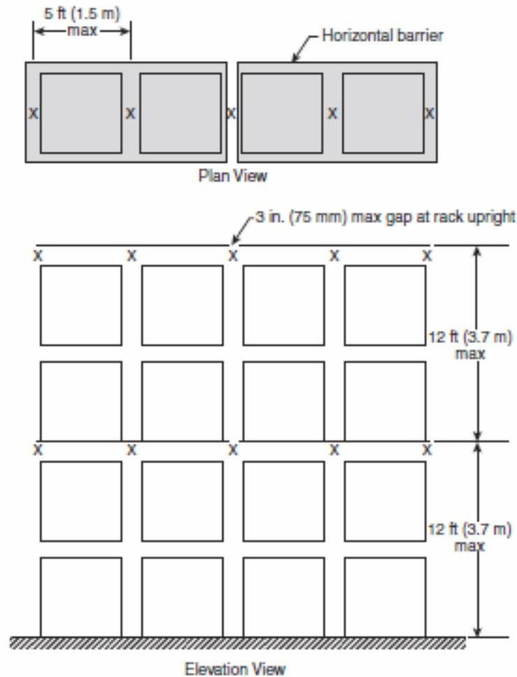
FIGURE 16.1.2.4.4.1(A) Alternative Protection for Single-Row Racks.
