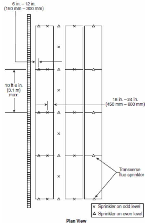
**FIGURE 20.5.6.4 Sprinkler Location and Spacing in Transverse Flues.**
