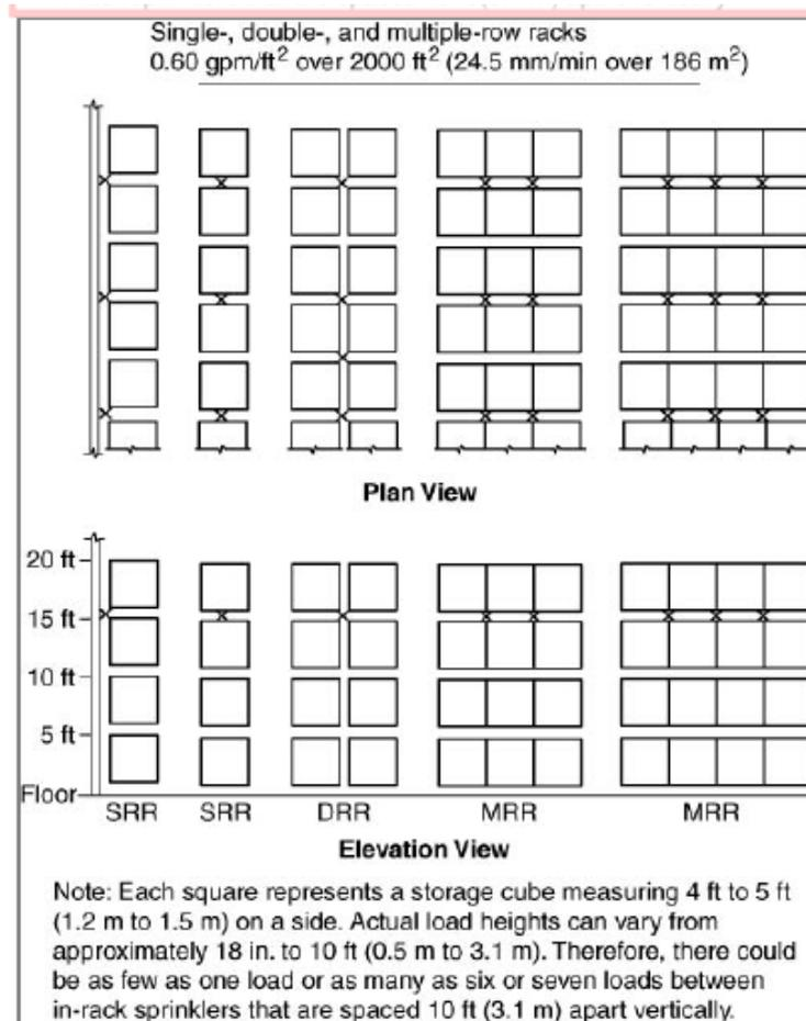
Figure 17.2.1.4(g) Exposed Nonexpanded Group A Plastics up to 20 ft in Height in up to a 25 ft High Building with One Level of Closely Spaced In-Rack Sprinklers.
